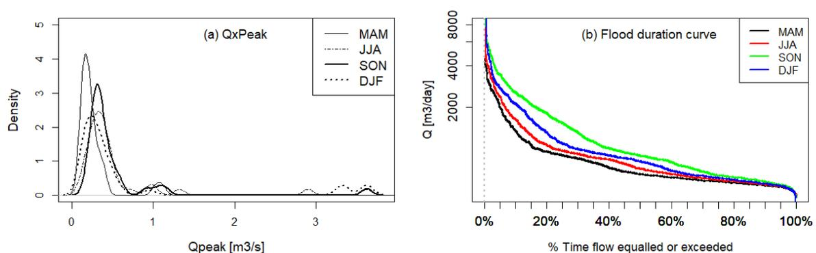
**Fig. 3: Characteristics of simulated stormwater in combined pipe at the outlet of the catchment: (a) by Kernel density estimates of QxPeak (monthly maximum of peak flow (m3/s)) and (b) as flood duration curves for daily flow.**
